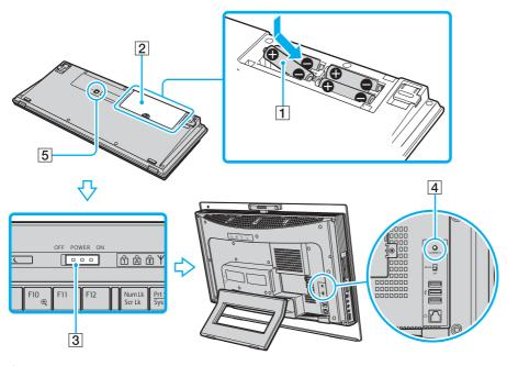
If the wireless keyboard does not operate properly, the batteries may need to be replaced. If the wireless keyboard is not being used for an extended period of time, remove the batteries to avoid possible damage from battery leakage.
